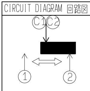
CONTACT SHALL BE POSITIONED AT ① OR ② IN DELIVERY.
